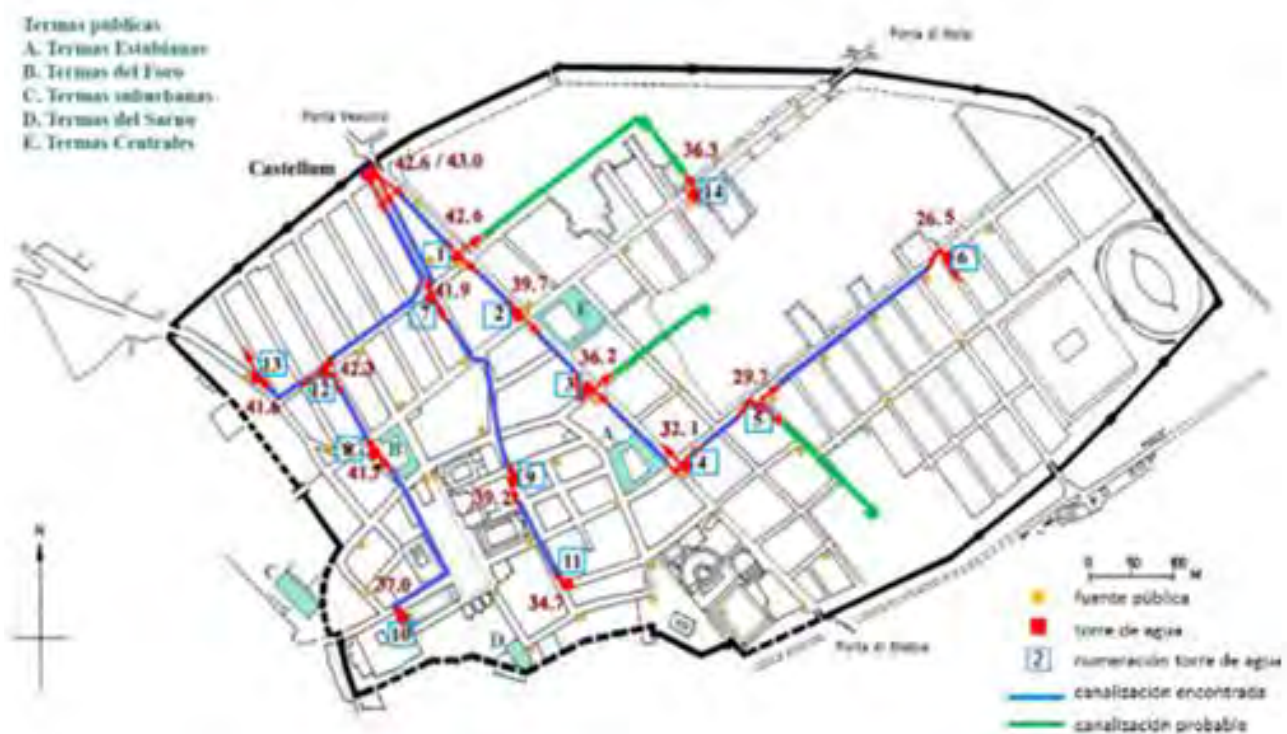
FIGURA 03 » Water distribution in the city of Pompeii, with its main elements and conduits. Prepared based on the work of OLSSON 2015:18, 91.
